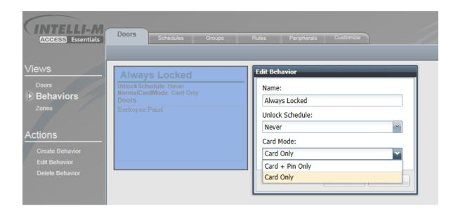
This will allow users to operate in a *Card Only* or *PIN Only* environment. Because the HID reader is an 8-bit burst reader, the PIN code is cached until the # key has been punched, and it subsequently sends the PIN Code to Intelli-M® Access. Therefore, Intelli-M® Access sees the PIN Code exactly like a Card Code.
